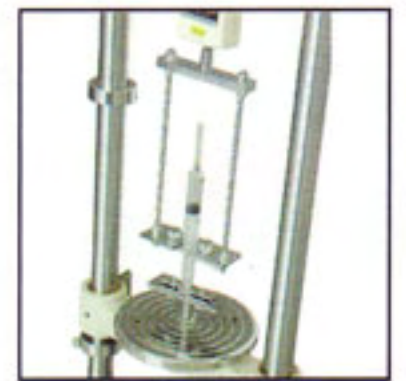
Test thrust & pull of injector
