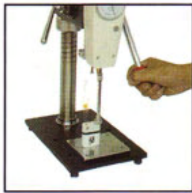
Test Pressure of Lighter
