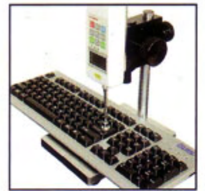
Test Pressure of PC Keyboard Button
